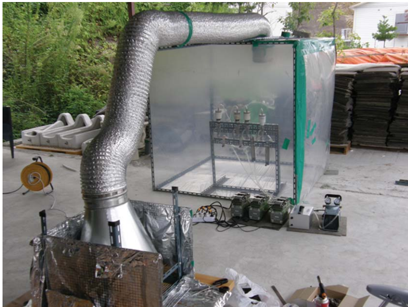
Fig. 1. Sampling system for meat cooking.
