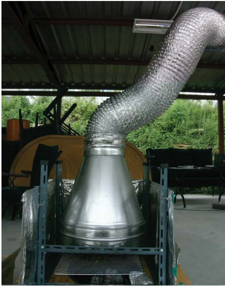
Fig. 2. Sampling system of spiced pork cooking.
