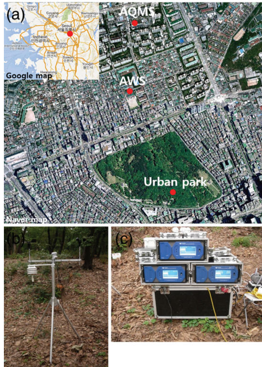
Fig. 1. (a) Satellite image including observation locations (Google map and Naver map), and photos of (b) a thermometer and an anemovane and (c) ozone and nitrogen dioxide analyzers installed in the Seolleung park.
