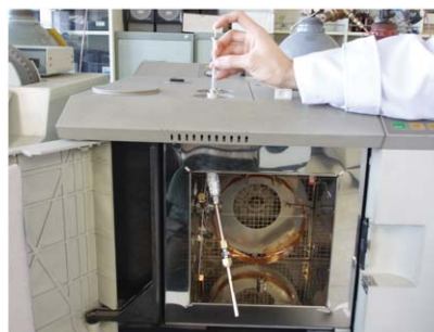
Fig. 3. Spiking of liquid standards onto adsorbent tubes through a GC packed column injector.
