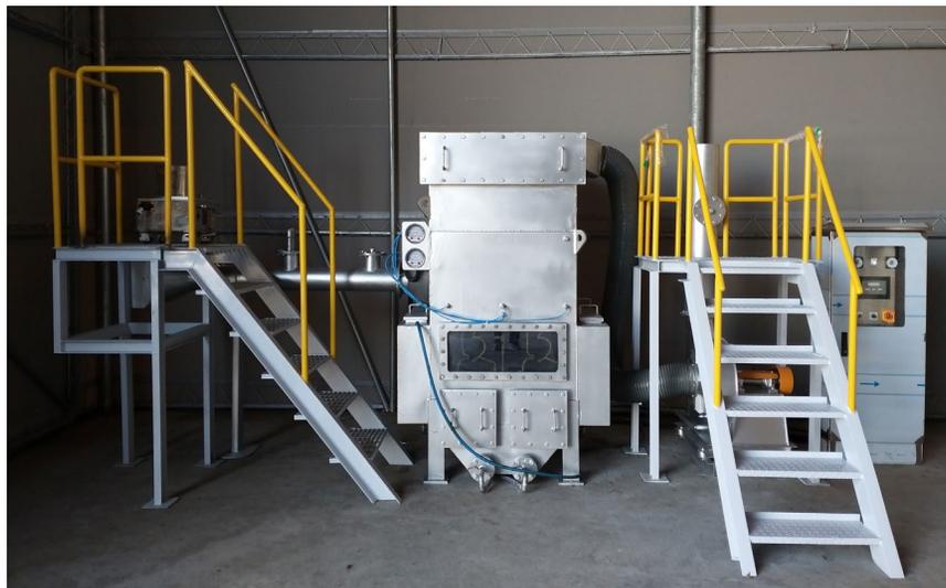
**Fig. 2.** Real image of pilot scale two-stage vortex scrubber.
