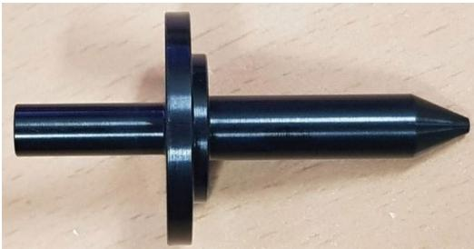
**Fig. 4.** The image of the single nozzle for an inertial impactor.
