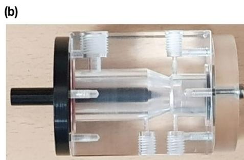
**Fig. 5.** The designed impactor plate and impactor plate housing ((a) impactor plate and (b) impactor plate housing).
