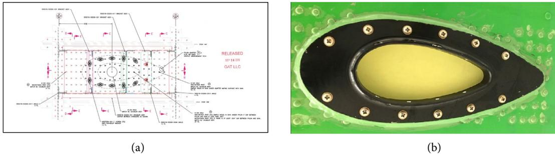
Fig. 6. (a) Drawing and (b) picture of the pylon adaptor.
