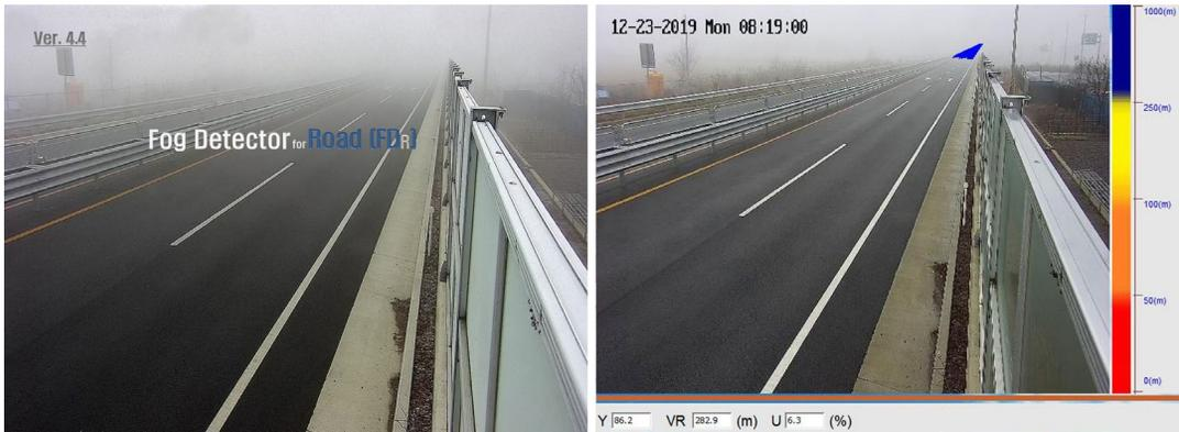
**Fig. 6.** Display result (right) of a fog detection area on the road by the fog pattern recognition method using the Fog Detector software program.
