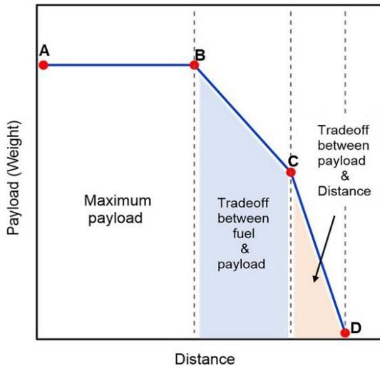
**Fig. 2.** Standard payload-distance diagram (Adapted from Ackert, 2013).
